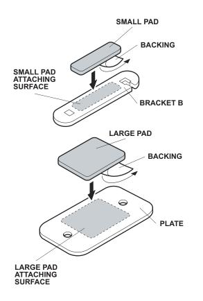
3. Using isopropyl alcohol on a shop towel, clean four plates where the large pads will attach. Remove the backing from the large pads and attach them to the plates.
